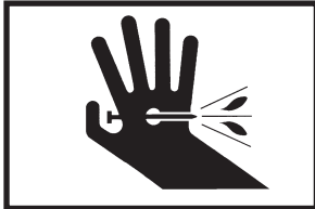
Never close tool with hand over fastener loading end of the tool. A serious hand injury from penetration by the piston or a discharged fastener could result.
